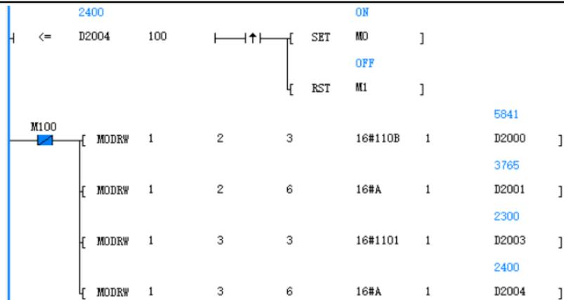
Figure 5.6 Programming case for RS485 communication
