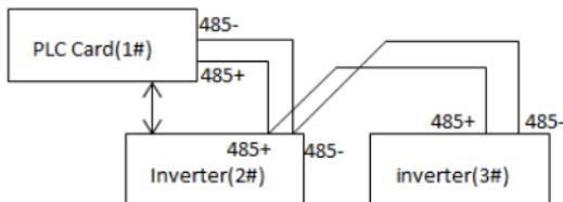
Figure 5.5 PLC card networking example
