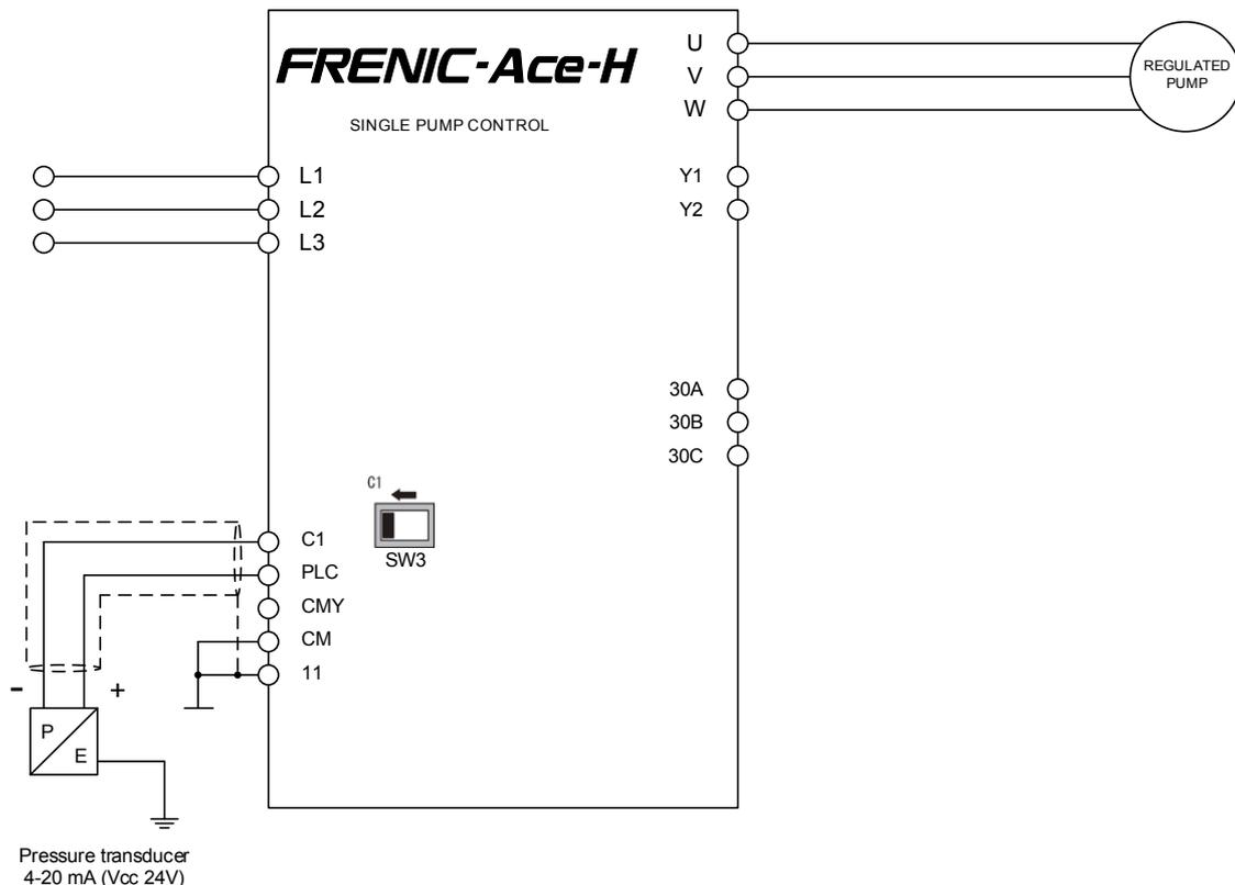
Figure 1.1: control schematic for 1 pump only
