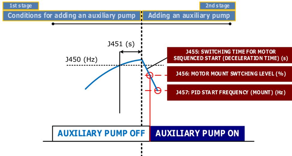
Figure 2.6: Auxiliary pump's connection
