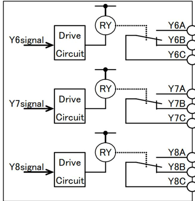
Figure 8.1 Internal Diagram OPC-F2-RY
