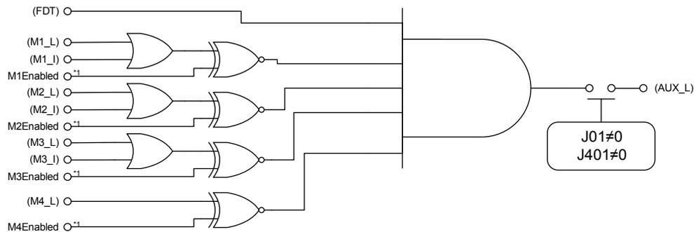
\*1 : This signal is generated by following diagram. (Internal signal)
