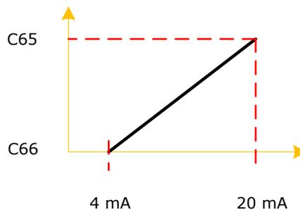
Figure 5.1: PID Display coefficients
