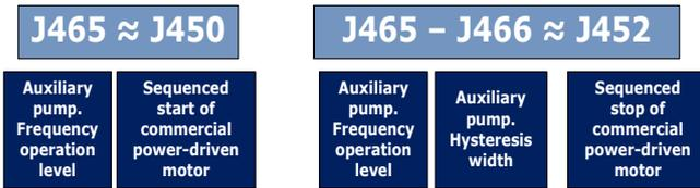
Using this control topology, it can be necessary to delay the disconnection of the motor from the commercial power supply (J453), in order to prevent the simultaneous disconnection of the auxiliary and the additional pumps. That is, the first pump to be disconnected should be the additional pump and then the auxiliary pump, but never at the same time.
