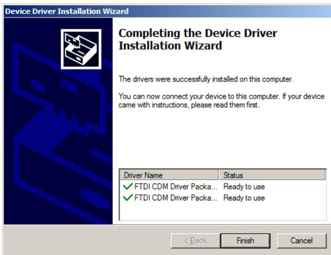
The actual setup of the driver in the computer is executed when connecting the PLC to the personal computer using a loader connecting cable. The progress of the setup is displayed on the bottom right of the computer screen.
