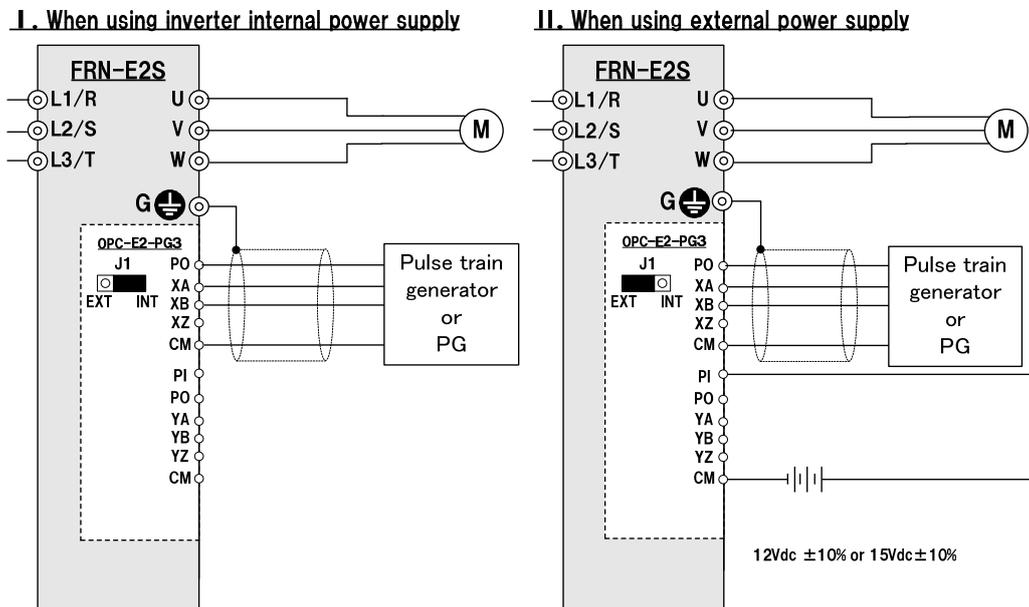
Figure 8 Connection Diagrams for Pulse Train Input
