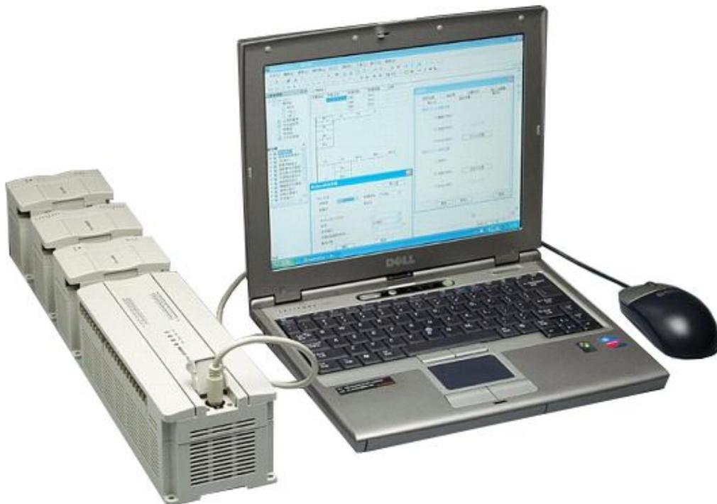
Figure 1-1 Connection of programming cable
