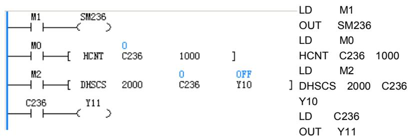
1. When M0 is ON, C236 will count in the interrupt mode when X0 changes from OFF to ON (see *错误! 未找到引用源。错误! 未找到引用源。* for the description of the X0 input frequency). When C236 changes from 999 to 1000, the C236 contact will be set. When C236 changes from 1001 to 1000, the C236 contact will be reset. When the C236 contact drives Y11, the execution of Y11 is determined by the user program scan cycle.
